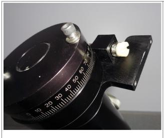
The plastic joint must be coupled with the aluminium one still fixed on the mount axis
