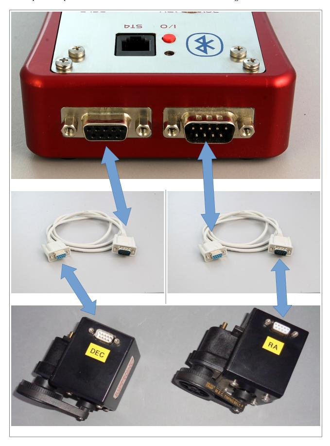
After the connection cables has been made, it is possible to power on the StarGo box and launch the StarGo Software (for the StarGo Software installation see StarGo User Manual and the Quick Start Guide).
