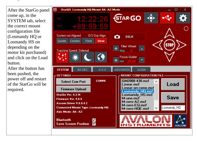
Now the StarGo it is configured to work with the Motor Kit and the mount. Before to use the mount, it is strongly suggested to read the StarGo User Manual.
