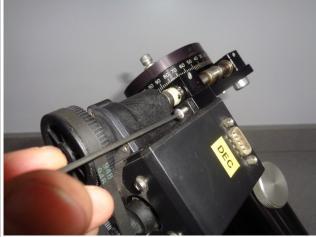
Now, by tightening the two screws available on the aluminium joint, it is possible to couple the motor kit with the corresponding mount axis.
