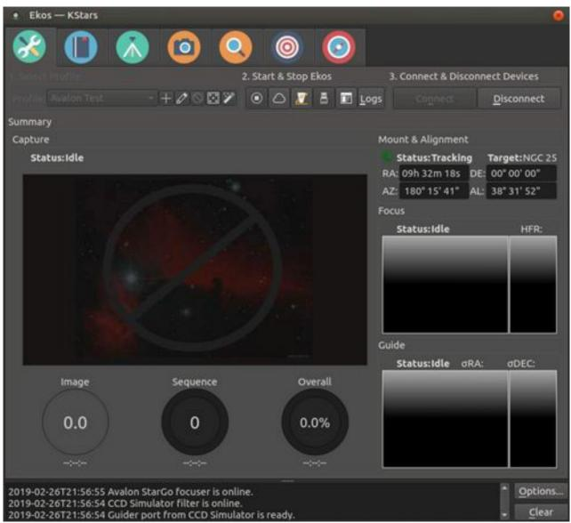
To control the telescope, it is necessary to open the operation window by clicking on the tab with the green tripod icon.
