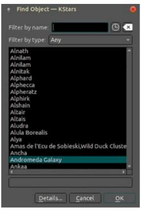
By double clicking the object name the chosen object is selected, the Find Object window is automatically closed and the Target field on the virtual keypad is populated with the catalog name of the object and its RA / DEC coordinates.
