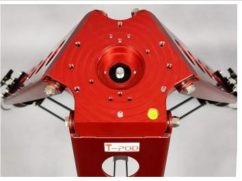
Then is possible to attach the UPAS on the T-pod, paying attention to make correspond the UPAS north side to the T-pod North leg. The antisliding screw must correspond to the dedicated slot hole.
